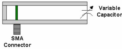
Figure 2: Geometry of SPA for reconfigurable antenna implementation.
