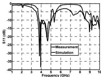
Figure 11: Comparison of measured and simulated results for fabricated three-stub tuner.
