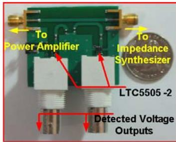
Figure 12: Photograph of the power detector combined with the three-line directional coupler.
