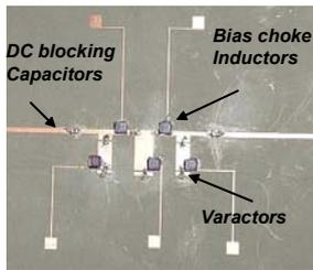
Figure 10: Photograph of three stub RF impedance tuner.
