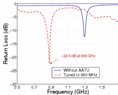
Figure 14: Narrowband tuning ability of the ATU. The SPA is tuned to 880 MHz.
