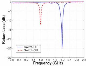
Figure 3: Measured return loss of the SPA tuned to two frequency bands.
