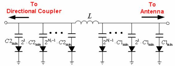
Figure 4: Impedance synthesizer configuration.
