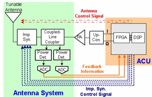
Figure 1: Block diagram of closed-loop automatic antenna tuning unit (ATU) for SDR transmitter.
