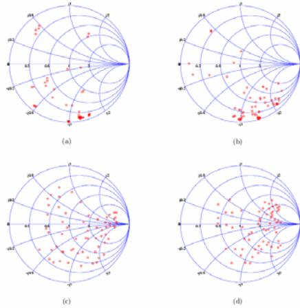
Figure 7: Measured matchable domains of the fabricated impedance synthesizer with 6 capacitors at (a) 800 MHz, (b) 900 MHz, (c) 1800 MHz, and (d) 1900 MHz.
