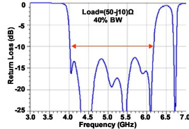
Figure 9: Simulated return loss of ten stub microstrip tuner.
