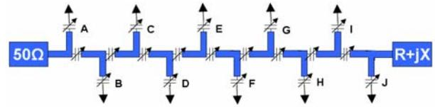
Figure 8: Ten stub reconfigurable RF impedance tuner.
