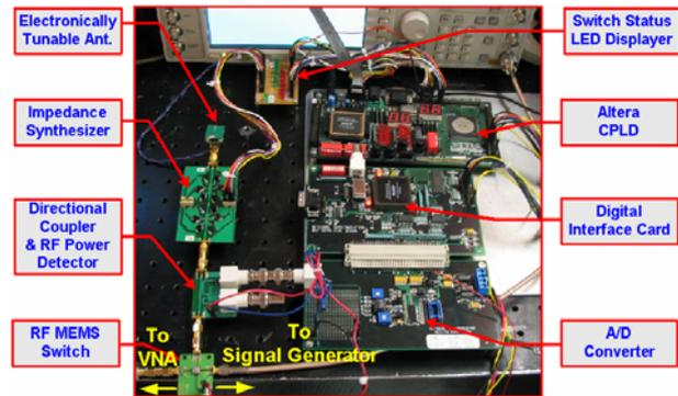
Figure 13: Photograph of the ATU demonstration setup.
