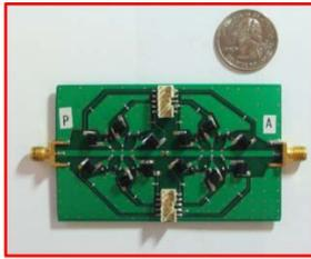
Figure 6: Photograph of the fabricated impedance synthesizer.
