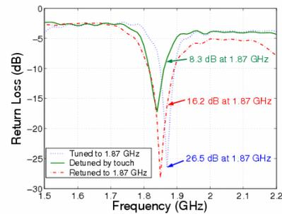
Figure 15: Automatic tuning ability of the ATU.
