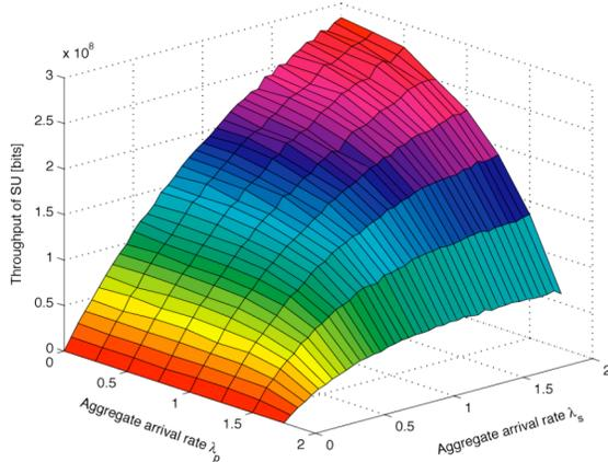
**Figure 6:** Random scheme, aggregate throughput for all SUs in [bits/s] as a function of aggregate SU and PU arrival rates  $\lambda_s$  and  $\lambda_p$
