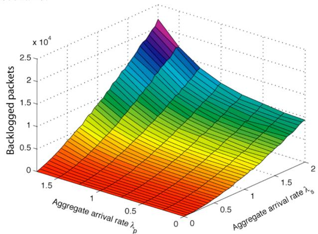
**Figure 5:** Random scheme, aggregate backlogged packets for all SUs as a function of aggregate SU and PU arrival rates  $\lambda_s$  and  $\lambda_p$ .
