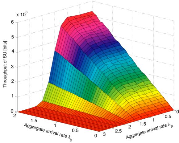
**Figure 4:** Assignment scheme, aggregate throughput for all SUs in [bits/s] as a function of aggregate SU and PU arrival rates  $\lambda_s$  and  $\lambda_p$
