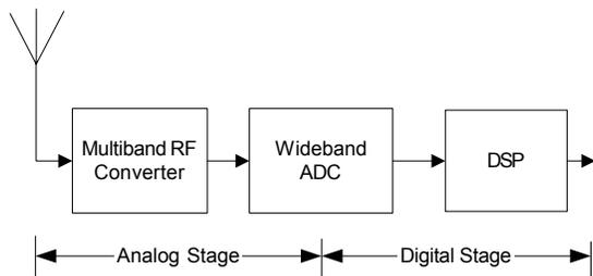
**Figure 1. Major Building Blocks of an SDR Device**
