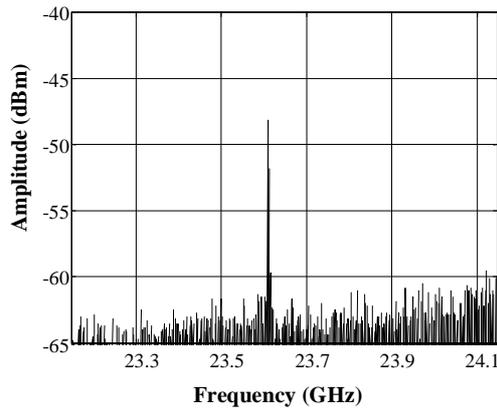
Figure 6: Microwave output of the dual-frequency ECL
