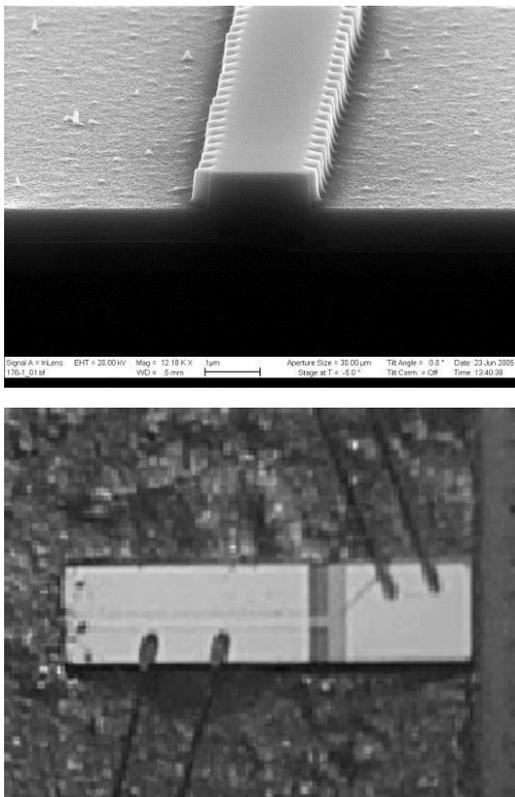
Figure 10: Elements of a photonic integrate circuit; the top image is a first-order grating etched in a waveguide, while the lower image is laser monolithically integrated with an electro-absorption modulator using Quantum Well Intermixing [9].
