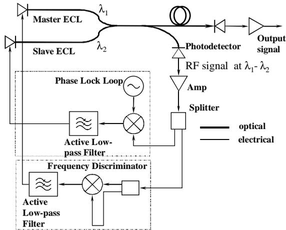
Figure 3: Schematic diagram for the optical PLL.
