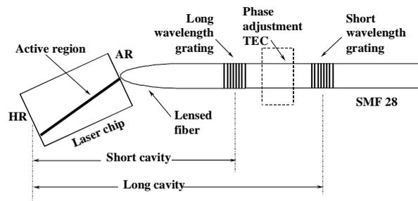
Figure 5: Schematic representation of the ECL. The laser chip has a high-reflectivity (HR) coating on one facet and an anti-reflection (AR) coating on the other. Each grating forms a cavity in the lensed fiber, with a phase adjustment section between them.
