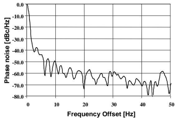
Figure 4: Optical PLL phase noise at an operating frequency of 11.224 GHz.
