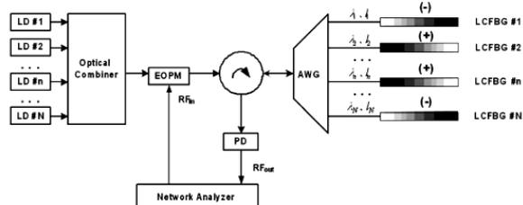
Figure 8: Basic architecture for the proposed optical RF filter.
