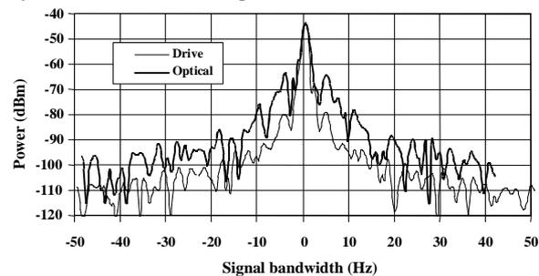
Figure 2: Comparison of the optically-generated 50 GHz signal (optical signal) to the 12.5 GHz electrical drive signal. Note that center frequencies have been normalized to allow comparison of the linewidths.
