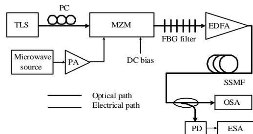
Figure 1: Experimental setup for optical generation mm-wave signals using the non-linearity of an optical modulator (TLS: tunable laser source, MZM: Mach-Zehnder modulator, EDFA: erbium-doped fiber amplifier, PA: power amplifier, OSA: optical spectrum analyzer, PD: photo-detector, ESA: electrical spectrum analyzer, SSMF: standard single mode fiber).
