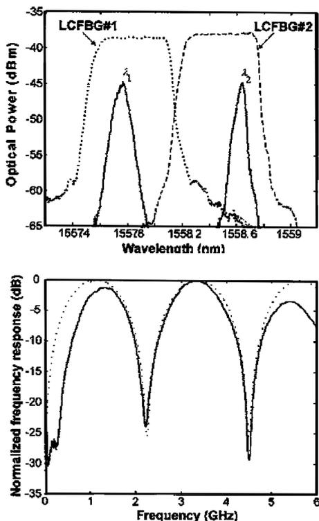
Figure 9: Experimental results of the two-tap filter with one negative coefficient. (a) Measured optical spectrum (solid curve) when  $\lambda_1$  is reflected by LCFBG#1 from the short wavelength port and  $\lambda_2$  is reflected by LCFBG#2 from the long-wavelength port. (b) Frequency responses: measured (solid curve) and simulated (dotted curve), showing a bandpass filtering with one negative tap.
