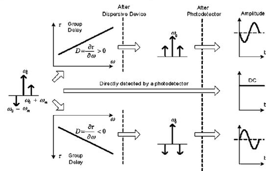
Figure 7: Illustration of the recovered RF modulating signals that sustain a positive, zero, or negative chromatic dispersion.
