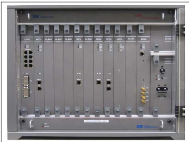
**Figure 1.** The developed MIMO receiver testbed
