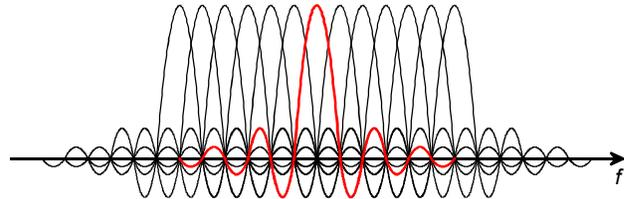
**Figure 1: Spectra of a group of sub-carriers in an OFDM signal.**
