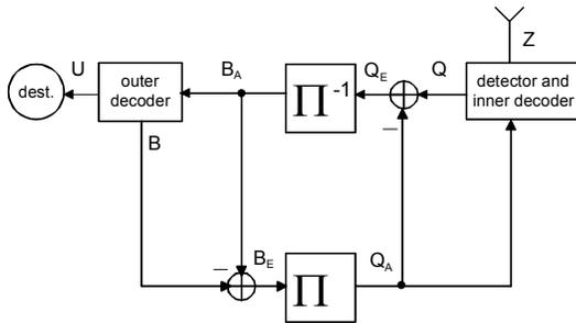
**Figure 5: Turbo decoder for a serially concatenated code.**
