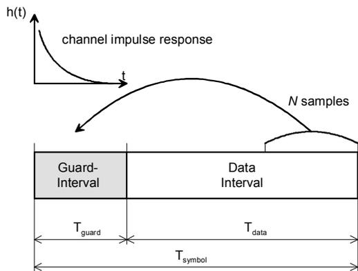
**Figure 2: Structure of an OFDM Symbol in time.**
