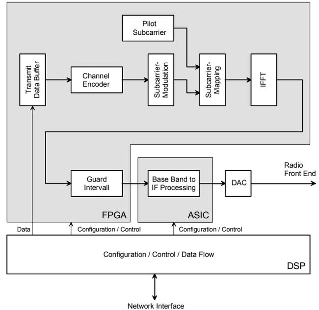
**Figure 6: Transmitter structure including which processing element performs which tasks.**
