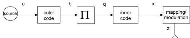
**Figure 4: Encoder structure for a serially concatenated code.**
