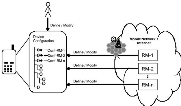
Figure 2: Decentralized Reconfiguration Control
