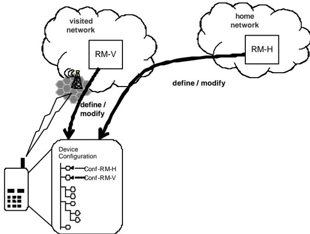
Figure 4: Autonomous Establishment of Reconfiguration Manager in a Visited Network
