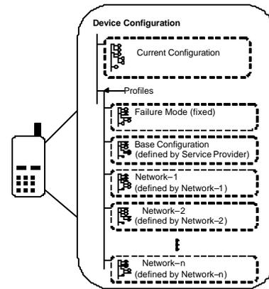
Figure 6: Automatically Established Network-specific Configuration Profiles
