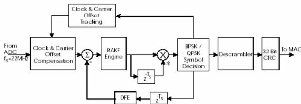
Figure 4: Block Diagram for 1 & 2 Mbps Receiver
