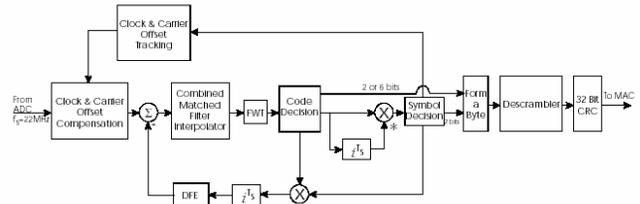
Figure 5: Block Diagram for 5.5 & 11 Mbps Receiver
