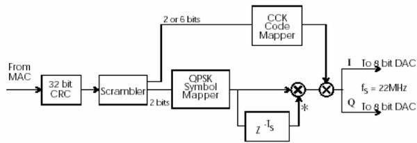
Figure 3: Block Diagram for 5.5 & 11 Mbps Transmitter
