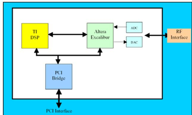
Figure 1: WLAN Reference Design Block Diagram
