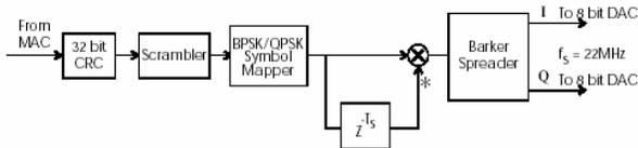
Figure 2: Block Diagram for 1 & 2 Mbps Transmitter
