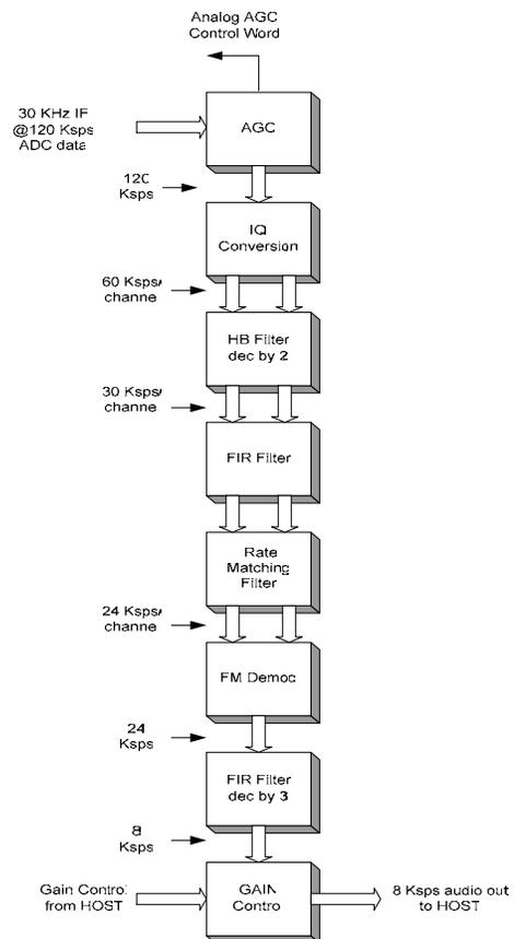
Figure 1- FM Receiver Block Diagram
