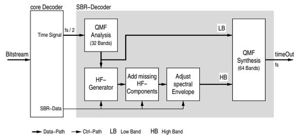
**Figure 2:** SBR decoder block diagram. The SBR-decoder operates as a post processor to the core decoder.
