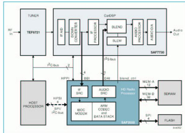
HD Radio - simplified system block diagram
