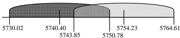
Fig. 2. Spectrum of test network (light gray) and interfering radio (dark gray). Frequency is in MHz.
