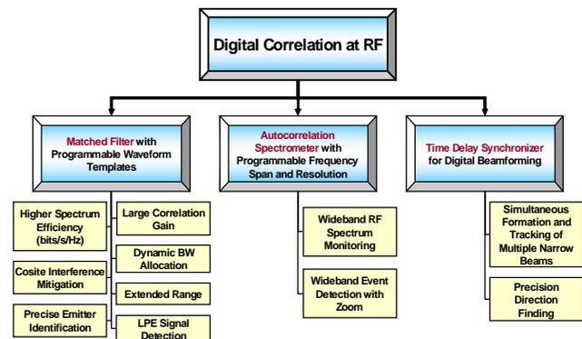
The novel features of this digital spectrometer are enabled by broadband, high-fidelity digitization and ultrafast (20-40 Gbps) digital processing of RF waveforms, using superconductor rapid single flux quantum (RSFQ) technology. Two central elements of such a digital-RF receiver, the ADC and the digital correlator, have already been demonstrated by HYPRES in the laboratory. The low noise, high linearity, and high dynamic range of the superconductor ADC permits high-fidelity
