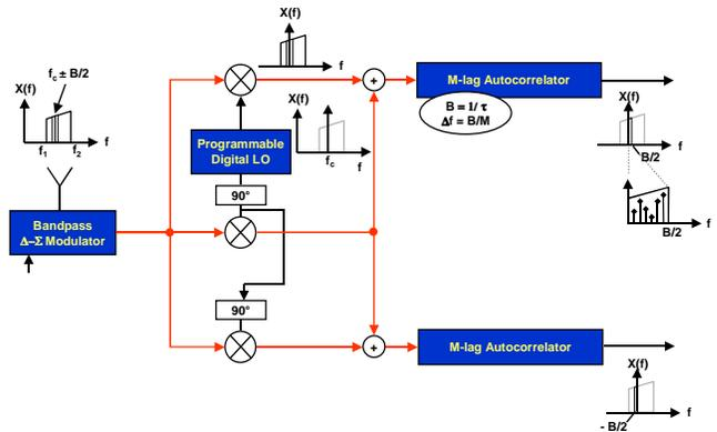
Figure 1. Autocorrelation spectrometer can choose a band of interest (of bandwidth  $B$ , centered around  $f_c$ ) within the receive band and resolve its spectrum with a resolution of  $B/M$ . The bandwidth and the center frequency are programmable. This allows one to monitor a wide band and then selectively examine narrower sub-bands with proportionately higher resolution.
