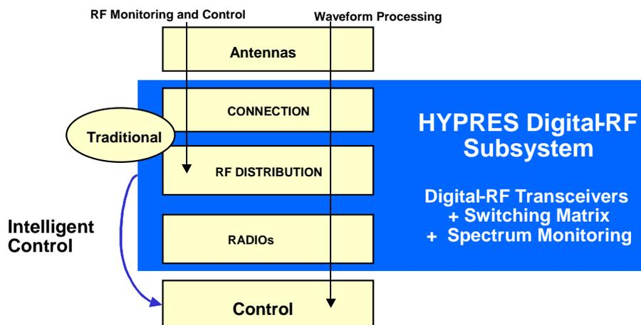
*A digital-RF subsystem, integrating the waveform processing function with real-time detection of the RF environment through a reconfigurable RF switching matrix for efficient spectral management, is shown in relation with the traditional RF communication system architecture.*
