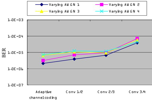
Figure 6. BER for each channel coding scheme at varying AWGN
