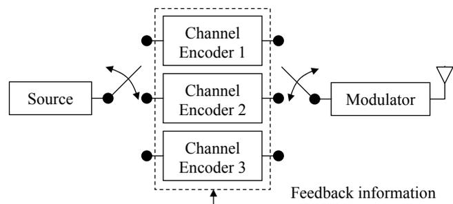
Figure 1. System model of transmitter
