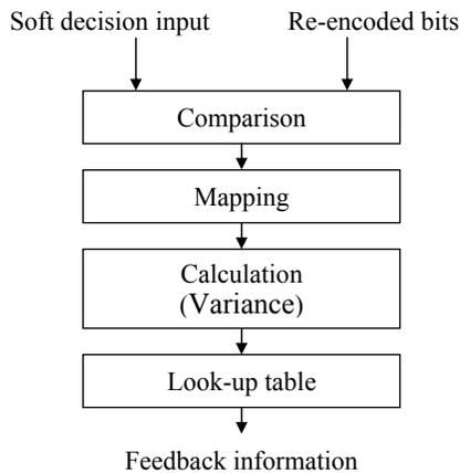
Figure 4. Procedure of channel quality metric
