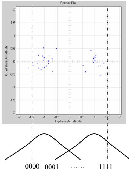
Figure 3. Soft decision input of channel decoder
