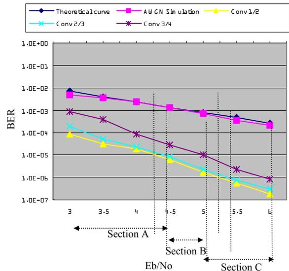
Figure 5. BER of convolution codes
