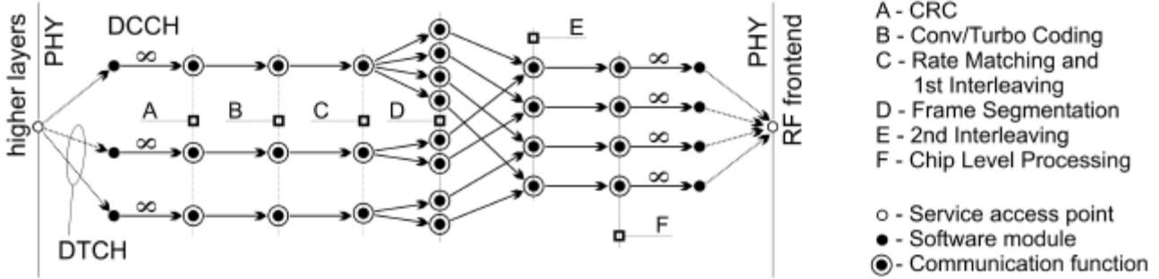
**Fig. 2:** Directed graph of an IMT-2000 W-CDMA transmitter, 64kbps uplink mode, abstracted from [6]
