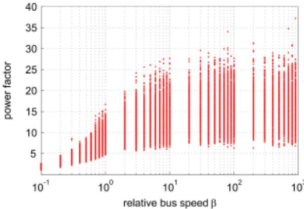
**Fig. 9:** Power factor for the pipelined co-processor subsystem
