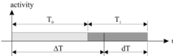
**Fig. 8:** Aggregate runtimes of co-processor ( $T_0$ ) and bus ( $T_1$ )
