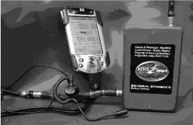
A small form factor prototype baseband module has been built. The circuit card measures 5 square inches, using 14 layers, .062 inch thick. Three power planes, three supply ground planes, two signal ground planes (analog and digital), and six signal layers provides the necessary isolation to minimize coupling between the RF and digital
