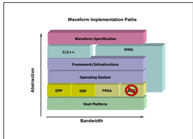
Figure 1: Software Radio Abstraction Layers
