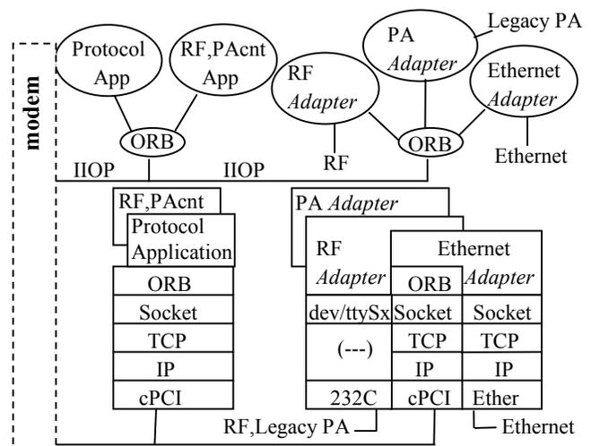
Figure 8. RF/PA Utility Application Block Diagram
