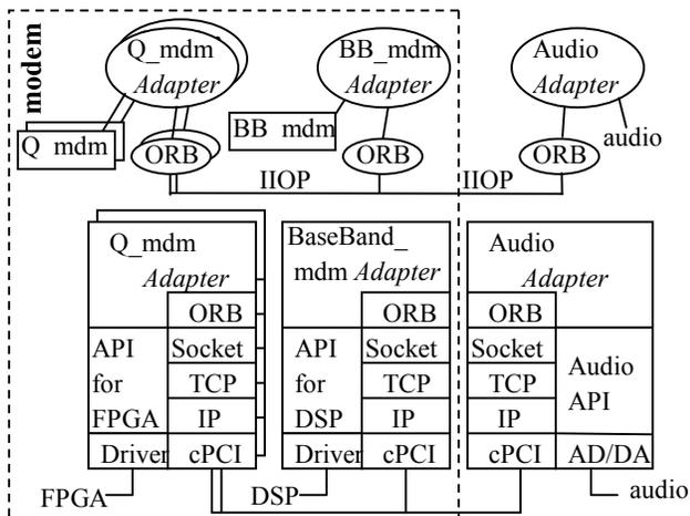
Figure 5. Voice Application Block Diagram
