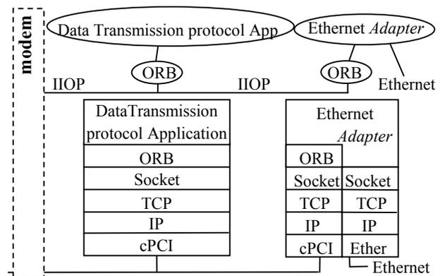
Figure 7. Data Transmission Application Block Diagram
