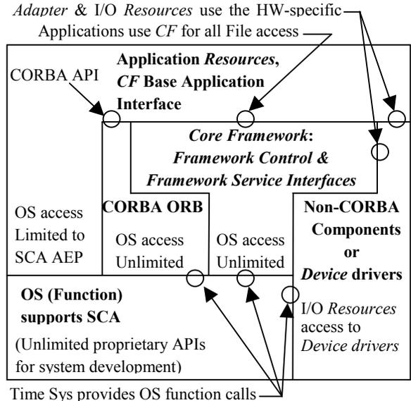
Figure 4. Relationship between OE and Application (No Device Interface is provided)
