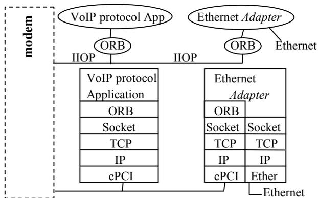
Figure 6. VoIP Application Block Diagram
