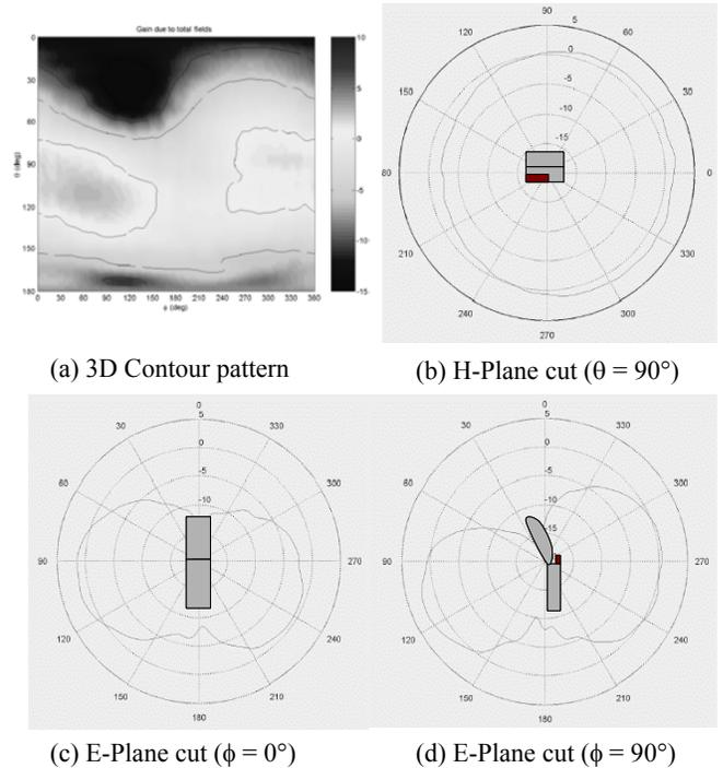
FIGURE 4. Radiation Pattern in GPS Band (1575 MHz)
