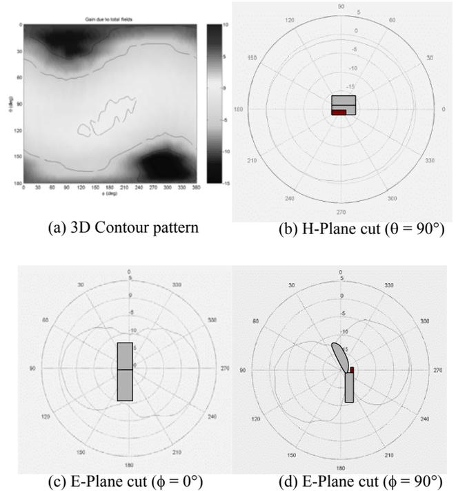
FIGURE 3. Radiation Pattern in CDMA Band (850 MHz)
