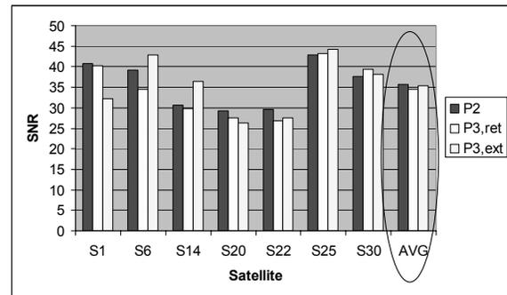
(c) Summary of the GPS active test (P2: Internal antenna, P3: Retracted whip antenna, P4, Extended whip antenna)
