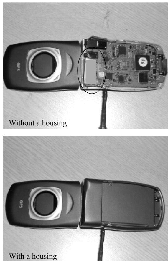
FIGURE 1. Antenna Installed in a CDMA/GPS Handset
