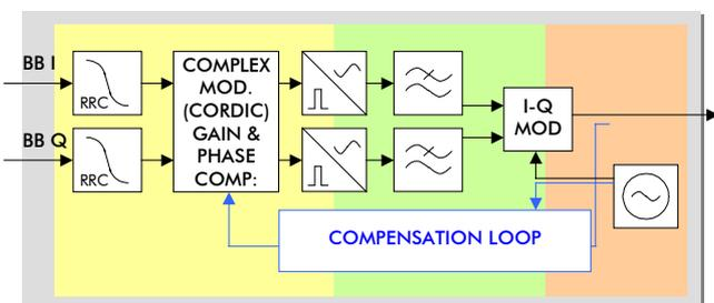
Figure 5: Architecture TX-Frontend
