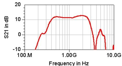
Figure 10: Bandwidth simulation of matched amplifier chip
