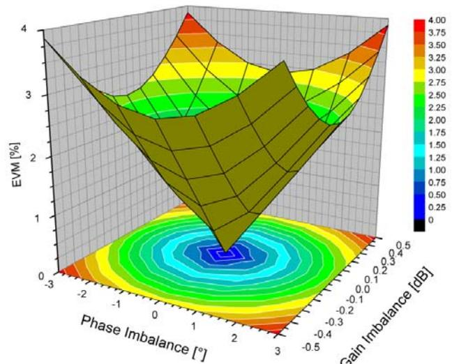
Figure 6: EVM over phase and gain imbalance in an analogue IQ-modulator
