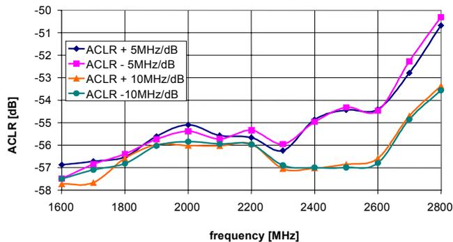
Figure 12: ACLR measurement results
