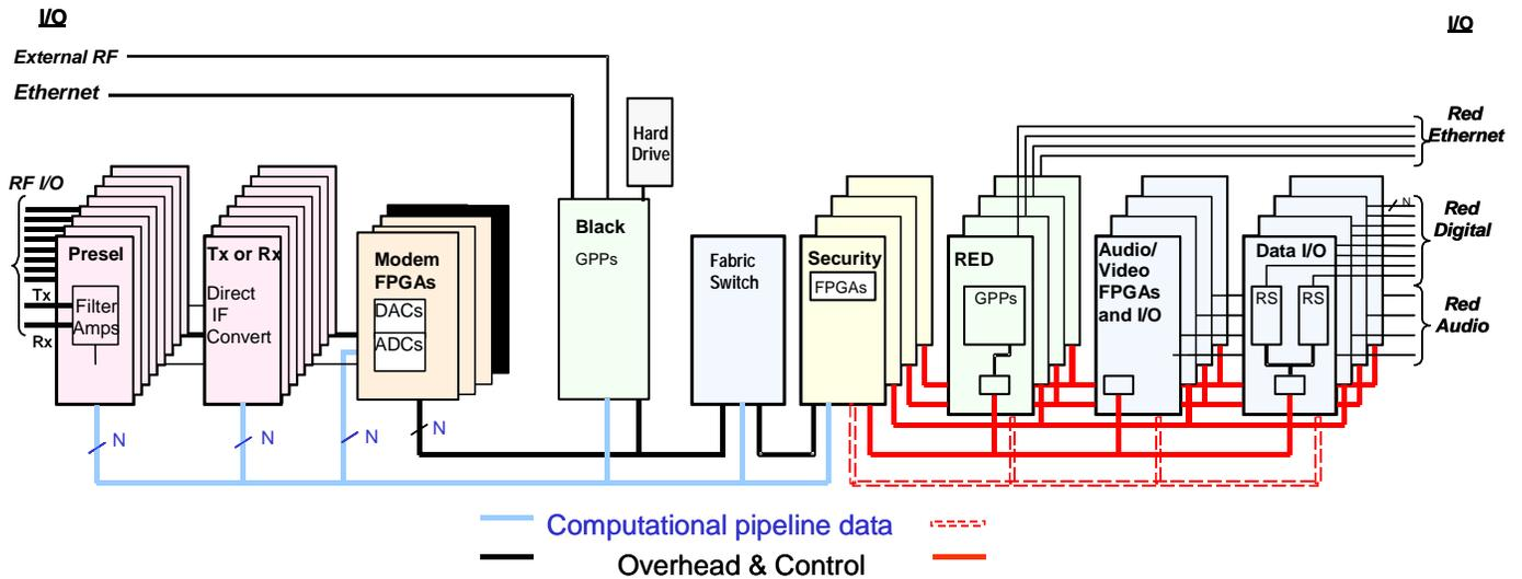
Figure 1. FPGA Based System Architecture.
