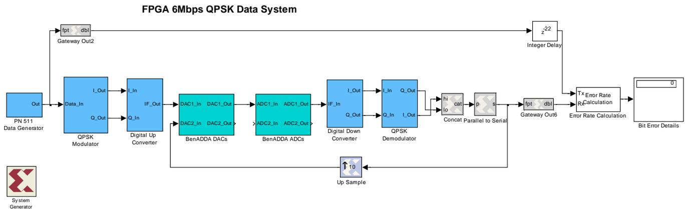
Figure 6. FPGA Based Waveform Model using Xilinx/Matlab Simulink Design Flow.
