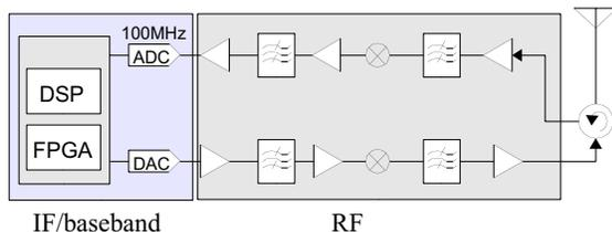
Figure 2: RF and IF/baseband interface in SDR
