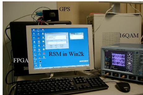
Figure 9: RSM prototype on a PC
