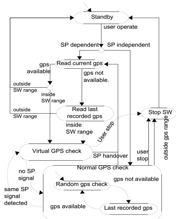
Figure 7: Stateflow of GPS checking scheme
