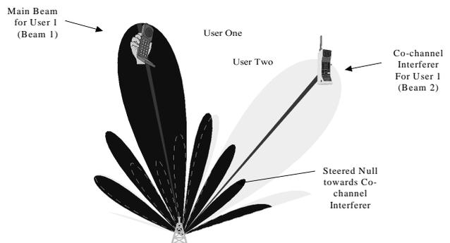
**Figure 3 – Adaptive Array Principles**
