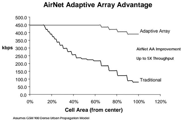
**Figure 7 – Adaptive Array Data Throughput**
