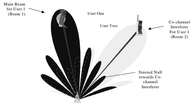
**Figure 3 – Adaptive Array Principles**
