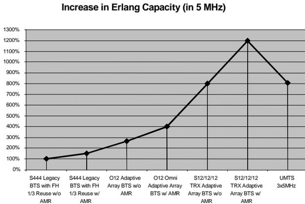
Figure 6 – Adaptive Array Capacity Comparison
