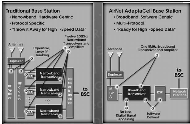
**Figure 1 – AdaptaCell BTS Architecture**
