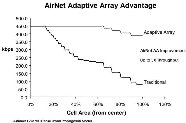
**Figure 7 – Adaptive Array Data Throughput**
