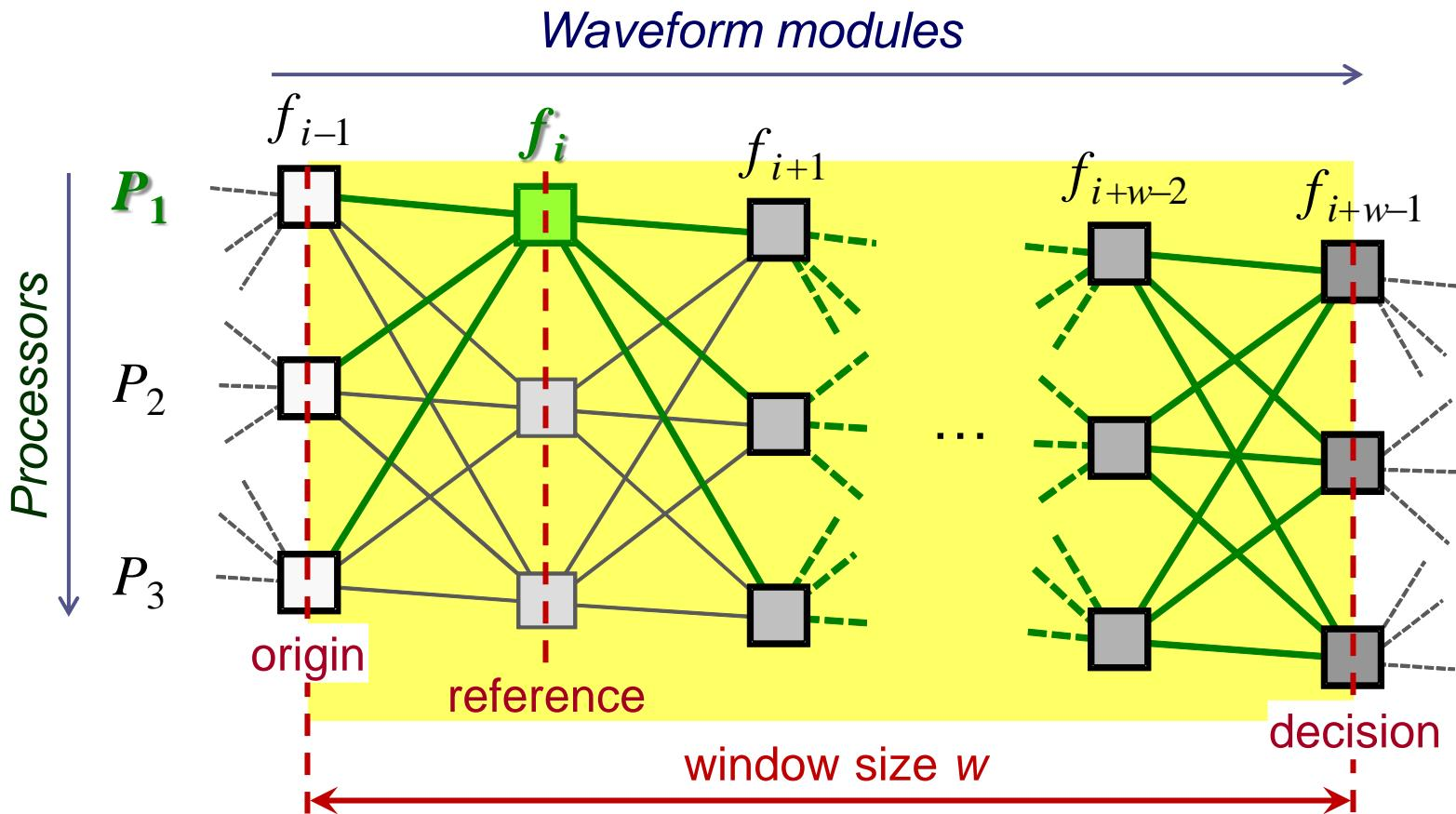
$\{P_1, f_i\}$  represents the mapping of waveform component  $f_i$  to processor  $P_1$
