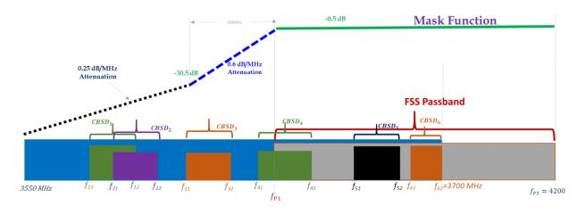
$f_{i1}$ : Lower edge of  $CBSD_i$ 's bandwidth  $f_{i2}$ : Upper edge of  $CBSD_i$ 's bandwidth
