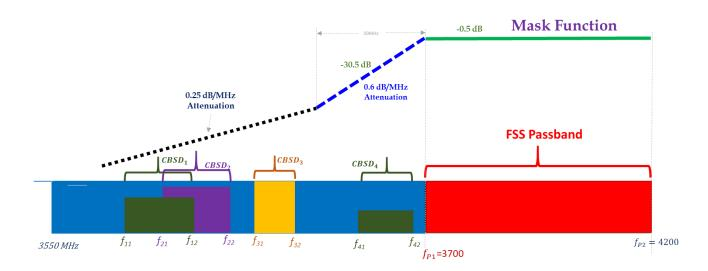
$f_{i1}$ : Lower edge of  $CBSD_i$ 's bandwidth  $f_{i2}$ : Upper edge of  $CBSD_i$ 's bandwidth
